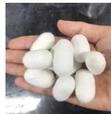
Fig. 3 Cellulose nanofiber reinforced cocoon of a silkworm.
