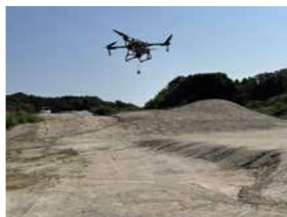
Fig. 2 Sphere falling test from drone at field simulating river channel blockage
