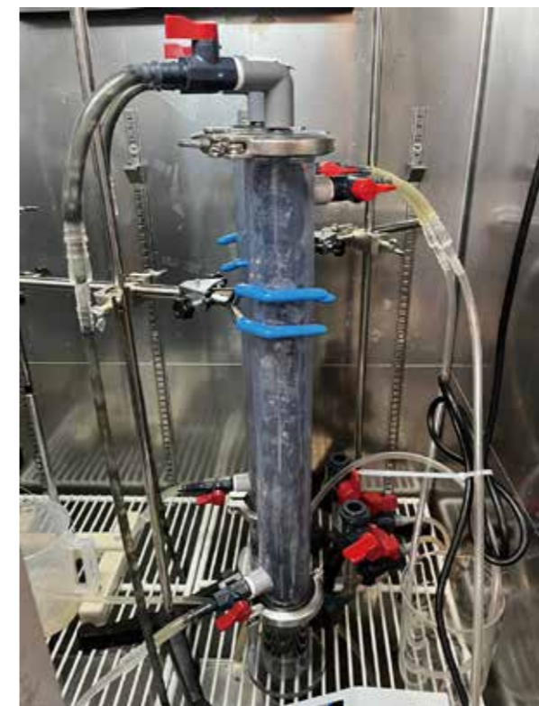
Photo 1. A DHS reactor removing nitrous oxide
