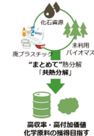
Fig. 3 Highly efficient utilization of carbon resources by the control of pyrolytic synergistic interactions during co-pyrolysis
