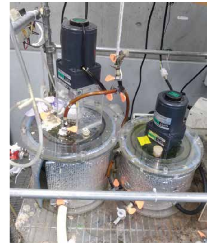
Photo 2. A laboratory-scale methane fermentation reactor treating duckweed.
