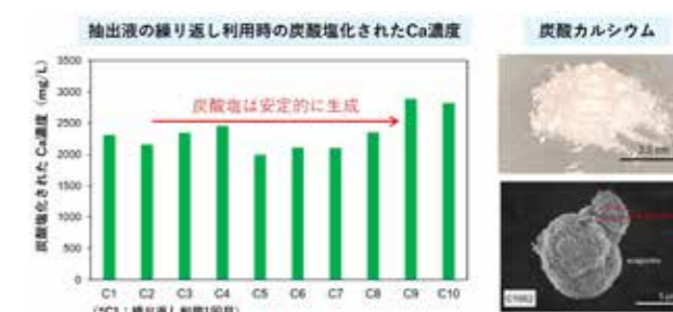
Fig. 4 CaCO 3 generated from concrete sludge cake via recycled use of a chelating agent solution.
