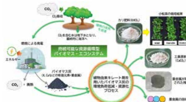
Fig. 3 Sustainable biomass power system integrating a resource-circulating ash treatment process.
