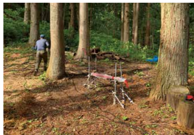
Fig. 2 Setting experiment of induction coils for geomagnetic measurements.
