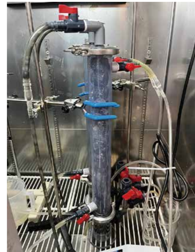
Fig. 1 DHS reactor treating nitrous oxide.
