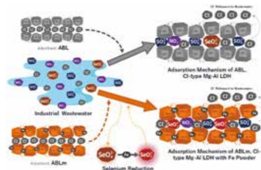
Fig. 2 Adsorption Mechanism of Se(VI) in industrial wastewater by ABL & ABLm.
