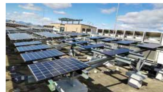
Fig. 3 Demonstration project to perform various tests on the secondary use of different types of solar panels at the rooftop of Tohoku University.
