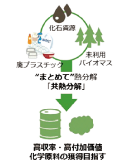
Fig. 4 Highly efficient utilization of carbon resources by the control of pyrolytic synergistic interactions during co-pyrolysis
