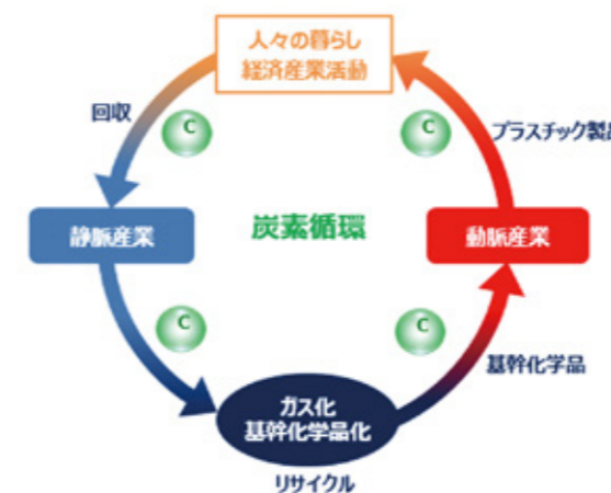
Fig. 3 Schematic illustration of carbon circulation system achieved by collaborating with arterial and venous industries.
