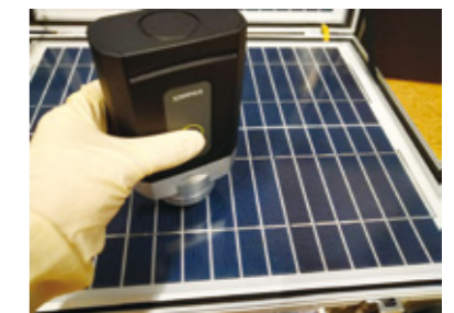
Fig. 3 Evaluation of solar panel with a near-infrared spectroscopy device
