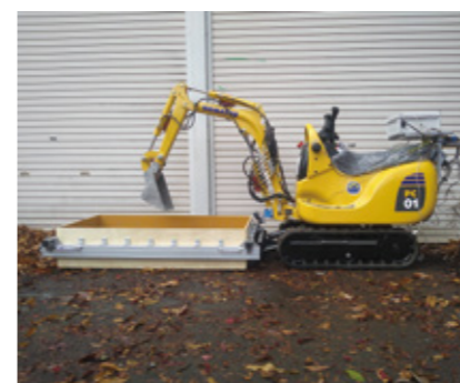
Fig. 4 Micro excavator equipped with various sensors
