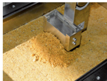
Fig.2 Blade excavation experiment
