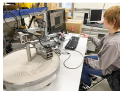
Fig.3 Apparatus for crawler turning
