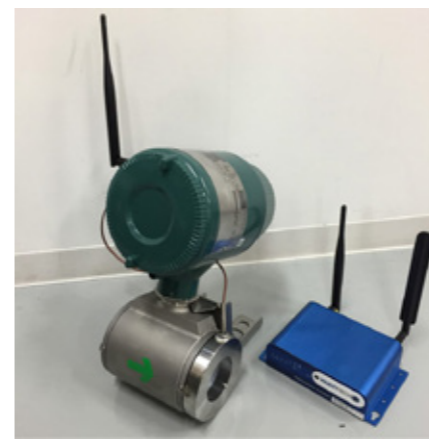
Fig.4 Remote monitoring system of hot springs for coexistence of geothermal power generation and hot springs
