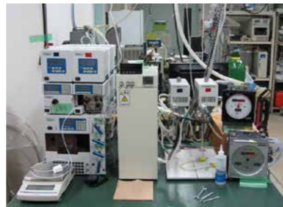
Fig.3 Flow-type subcritical fluid separation apparatus
