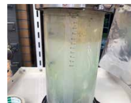
Fig.5 Hydrogen mixed gas production experiment using acidic hot spring water and aluminum scrap waste.
