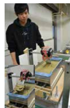
Fig.4 Bucket excavation experiment of the soil in water
