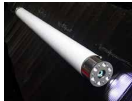
Fig.5 A prototype of borehole scanner for geothermal wells
