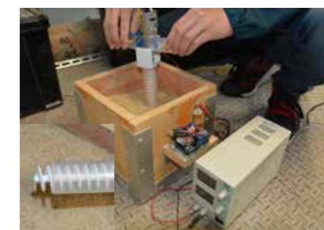
Fig.6 Screw type soil sampling device
