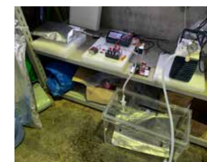
Fig.6 Driving experiment of hydrogen fuel cell using generated hydrogen mixed gas.
