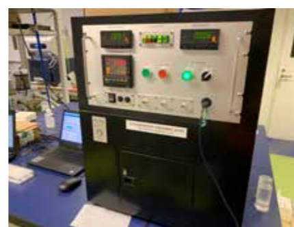
Fig.3 Developed TL measuring equipment for commercial use.
