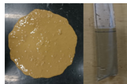
Fig.3 Flowability test (left) and bleeding test (right)
