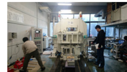
Fig.5 Novel high-temperature true triaxial hydrofracturing experimental system
