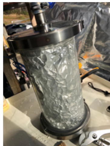
Fig.2 Hydrogen production through aluminum-hot spring water reaction in the Tamagawa hot springs
