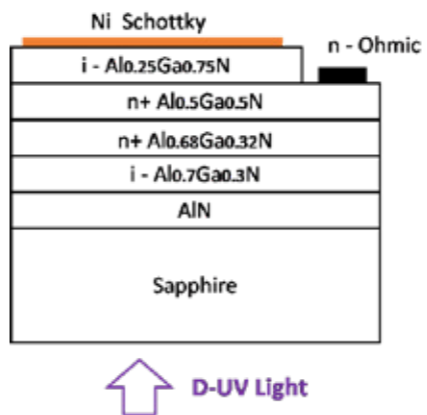
Fig.3 Device structure of the 310nm photodetector.
