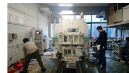
Fig.5 Novel high-temperature true triaxial hydrofracturing experimental system
