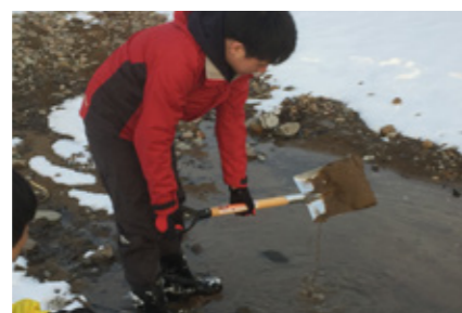
Fig.2 Sampling of high water content sludge
