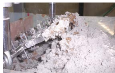
Fig.2 Laboratory test for mixing fiber-premixed cement and high-water content mud with different mixing blades.
