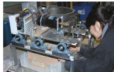
Fig.1 Developed apparatus to continuously recycle high-water content mud generated from disaster sites.
