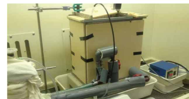
Fig.2 Ni electroplating equipment.
