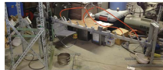
Fig.5 Experimental apparatus to separate soil from crushed asphalt under grizzly with a vibration mechanism.
