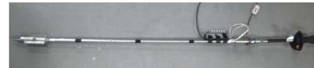
Fig.4 Developed test device composed of cone, vane and earth pressure gauge to estimate soil shear strength property.
