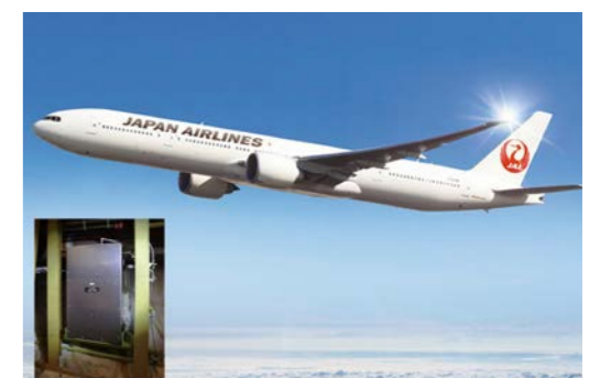
Fig. 3. Boeing 777-300ER aircraft and the Continuous CO 2 Measuring Equipment to be installed in her cargo room.
