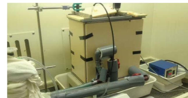
Fig.2 Ni electroplating equipment.
