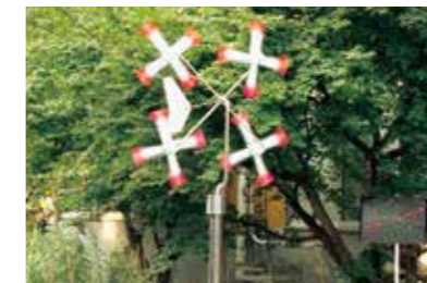
Fig.4 Dragonfly-windmills generating electric power for LED lamps.
