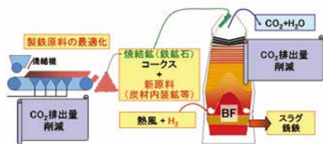
Fig.1 Methods of reducing CO 2 emission from ironmaking process.
