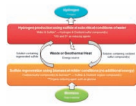
Fig.1: Hydrogen production from biomass via the sulfur redox cycle.
