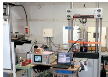
Fig. 1 Triaxial pressure vessel and experimental system developed for measuring poroelastic constants.
