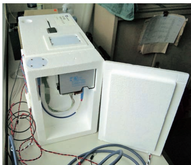
Fig. 2. New optical ozone sensor with small spectrometer.
