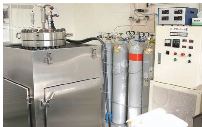
Fig. 2 Experimental apparatus for reduction of iron ore - carbon composite under high pressure.
