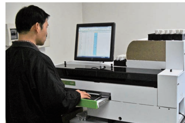
Photo3 Gamma-ray counter Wizard 2480 for measurement of radioactive materials
