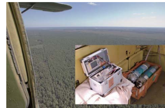
Forest in West Siberia and CO 2 measurement device onboard the aircraft.
