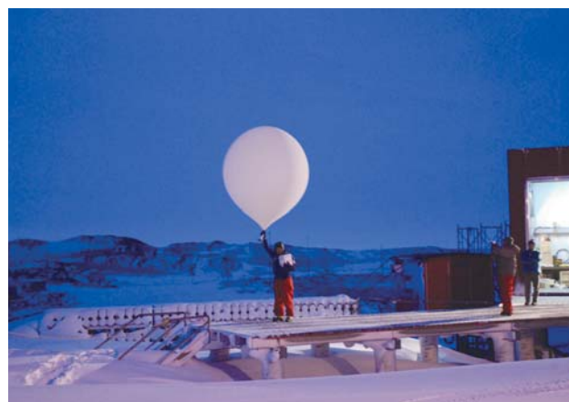
Ozonesonde launch at Syowa Station, Antarctica (69S, 40E) in polar night June, 2007.
