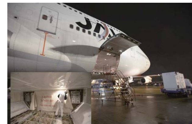
Boeing 747-400 and two equipments for atmospheric observation installed in her cargo room.
