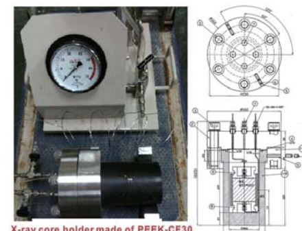
Fig. 7 Newly developed X-ray core holder made of a carbon fiber reinforced PEEK (PEEK-CF30).
