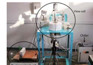
Fig. 9 Newly developed experimental system for phase behaviors in water/heavy oil systems.
