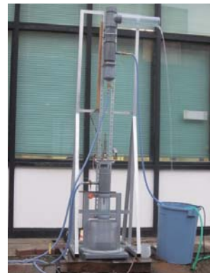
The developed experimental apparatus to measure durability for erosion of soil materials by using a jet flow in water.
