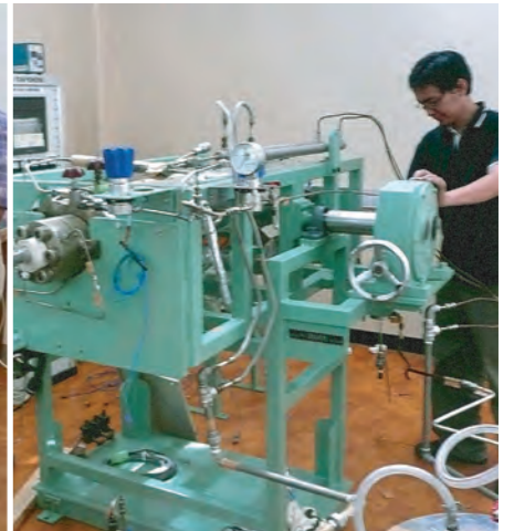
An experimental apparatus for the hydrothermal conversion of organic materials in laboratory.
