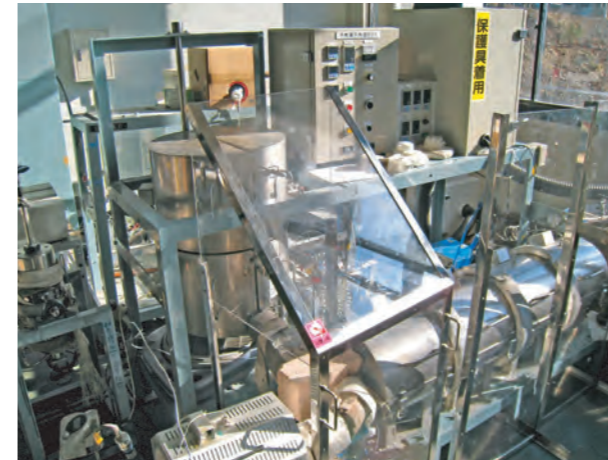
Figure 1 Continuous flow reactor for partial upgrading of bitumen by hydrothermal reaction.
