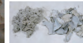
Crushed material (left) and paper of waste gypsum board (right).
