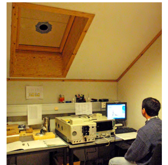
Fig.5. FTIR instrument set in AWI observatory
