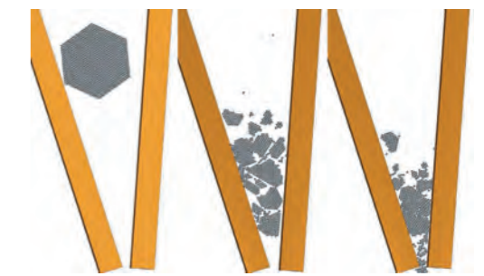
A simulation result of crushing with a mobile crusher.
