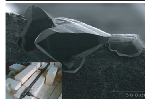
fig.6 流通式実験装置における石英析出の様子 Quartz deposition by hydrothermal experiment using flow-through type autoclave.
