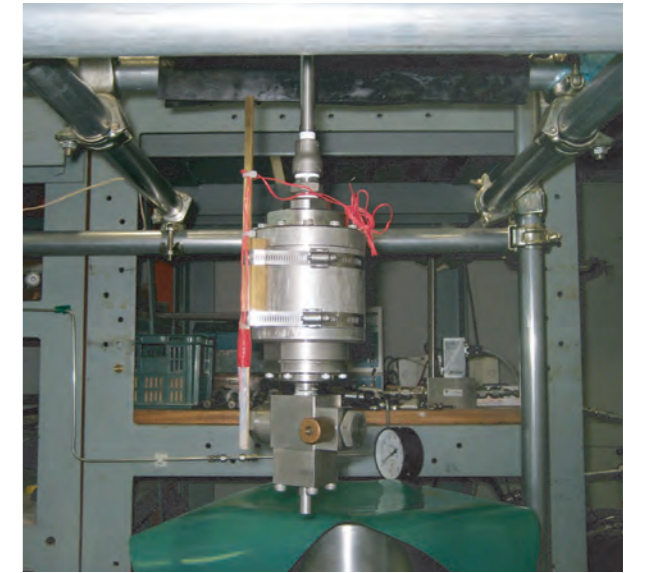
Self-rotating nozzle for removal of geothermal scale.
