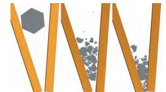
A simulation result of crushing with a mobile crusher.
