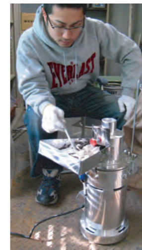
Crushing the paper of waste gypsum board with a hummer mill.
