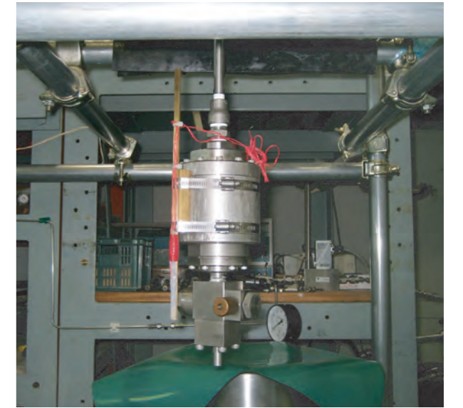
Self-rotating nozzle for removal of geothermal scale.
