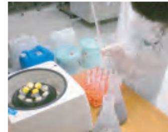
Leaching test of fluorine from the high fluoride-content sludge
