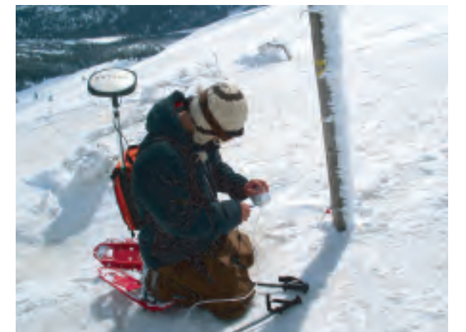
Snow depth measurement by GPS
