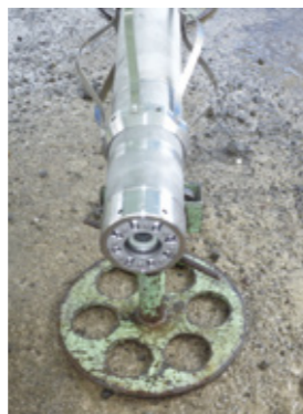
Fig. 2 BHS for geothermal wells
