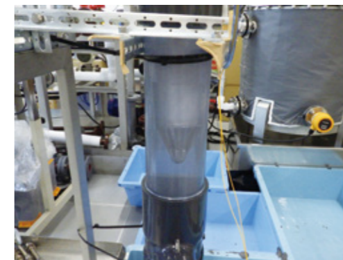
Fig. 5 Laboratory test of a fiber optic downhole flowmeter
