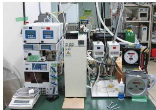
Fig. 3 Flow-type subcritical fluid separation apparatus
