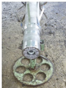
Fig. 2 BHE for geothermal wells
