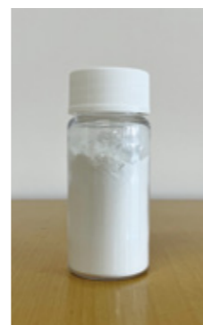
Fig. 3 Calcium carbonate produced by mineral carbonation technology
