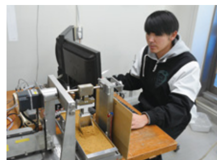
Fig.1 Apparatus for bucket excavation
