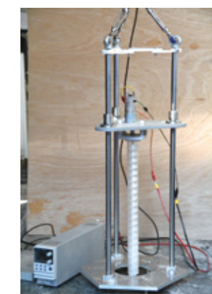
Fig.6 Screw type soil sampling device
