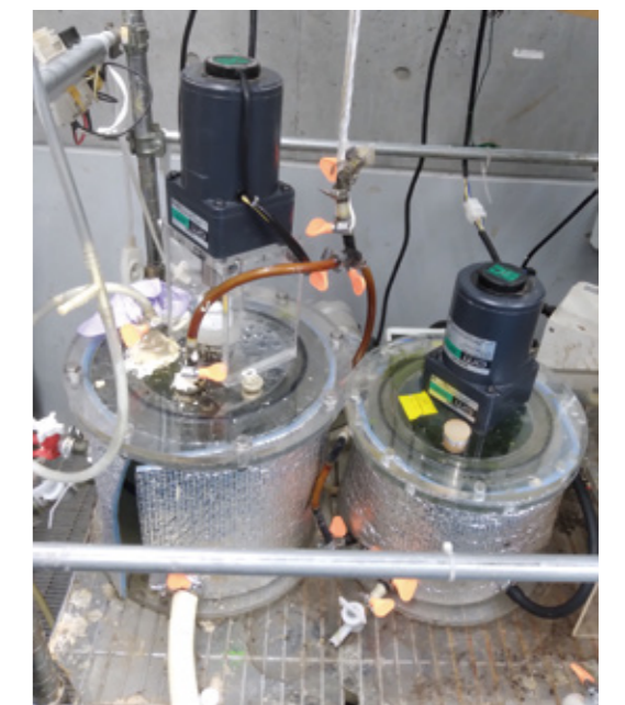
Fig.2 A laboratory-scale methane fermentation reactor.
