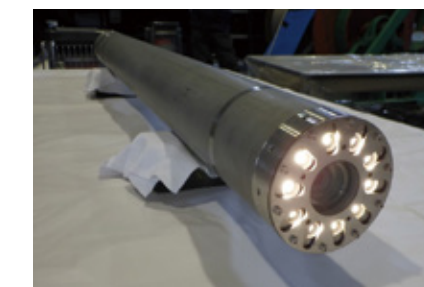
Fig.6 Scanning head of borehole scanner for geothermal well
