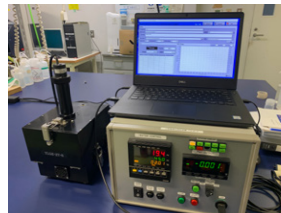
Fig.2 Developed small type TL measuring equipment.
