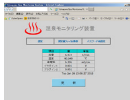
Fig.5 Data of hot spring transferred through internet
