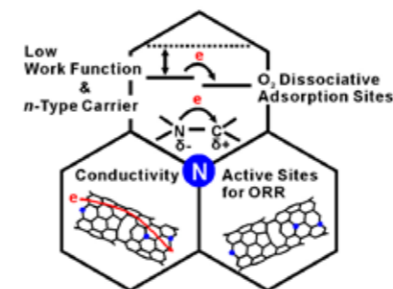
Fig.3 Tuning factors for efficient ORR catalytic activity of nitrogen-doped carbon materials.
