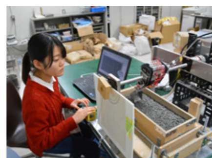
Fig.3 Bucket excavation experiment of crushed rocks
