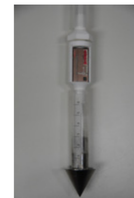
Fig.5 Cone with impact accelerometer
