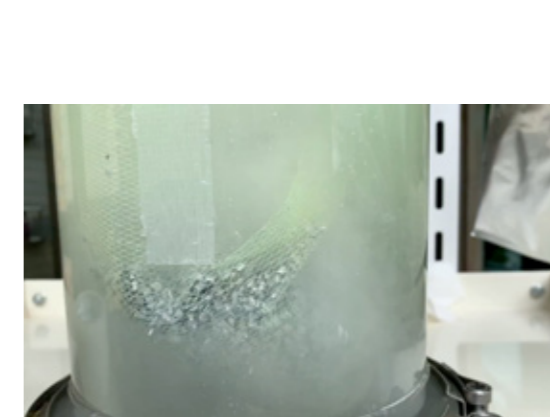
Fig.5 H 2 production (bubbles) using waste Al chips and Tamagawa hot spring water
