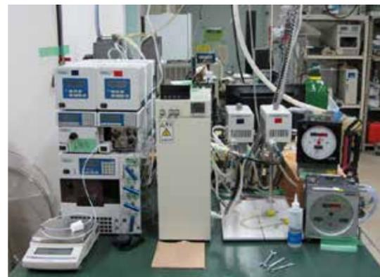
Fig.3 Flow-type subcritical fluid separation apparatus
