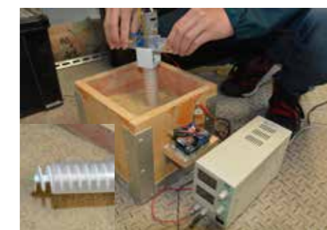
Fig.6 Screw type soil sampling device
