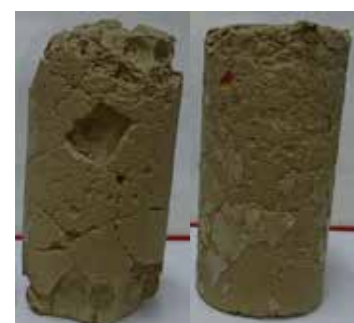
Fig.1 Specimens after 20th cycle of drying and wetting cyclic test (Left: without fiber, right: with fiber)
