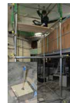
Fig.5 Cone falling experiment to predict ground strength
