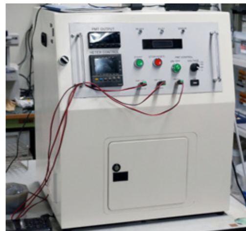
Fig.4 TL measuring equipment developed by SATREPS project.
