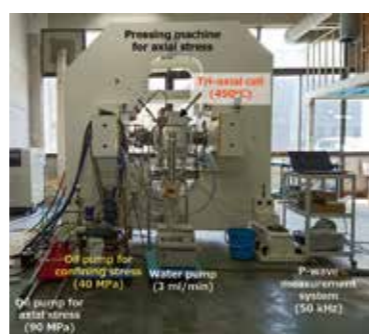
Fig.3 Large-scale hydraulic fracturing experiment under supercritical condition.
