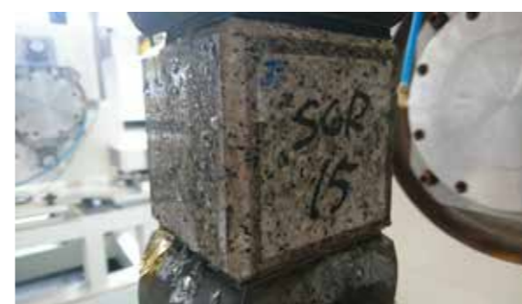
Fig.4 Permeability test after the hydraulic fracturing under over 400°C
