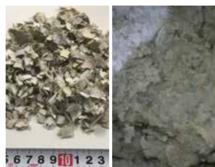
Fig.2 Board paper (left) and failure plane of modified soil by board paper (right)
