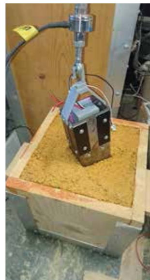
Fig.4 Soil sampling test using developed device
