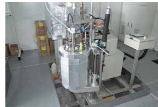
Laboratory test system of hydrogen production system using hot springs
