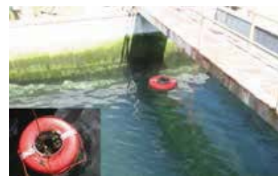
Fig.1 A filed trial of leachate treatment by Arabidopsis halleri ssp., in which a closed-up photo of hydroponic cultivation is in bottom left.
