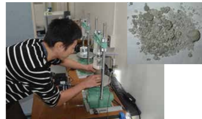
Fig.6 Measurement of strength property of Fiber-cement stabilized soil including granule (upper right side picture)
