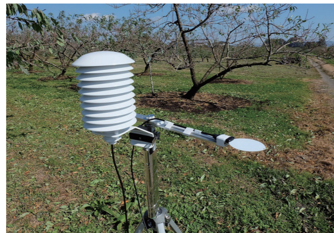
Fig.2 Meteorological observation using the leaf wetness sensor
