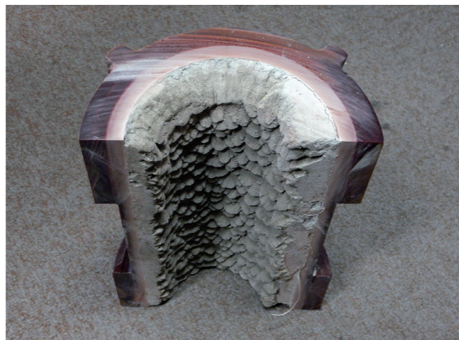
Fig.2 Pipe with Talc scale 3 month elapsed.
